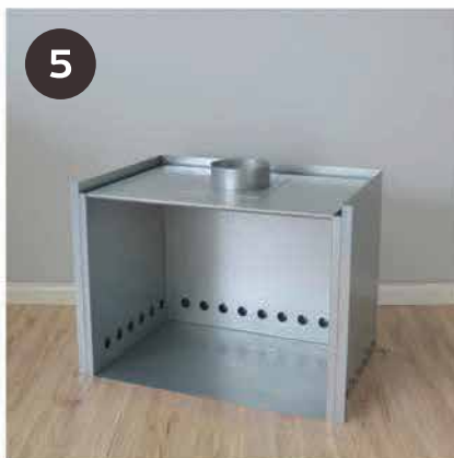
5 Screw outer left, outer right and outer rear panels in place with vent holes to the bottom, returns facing outwards.
